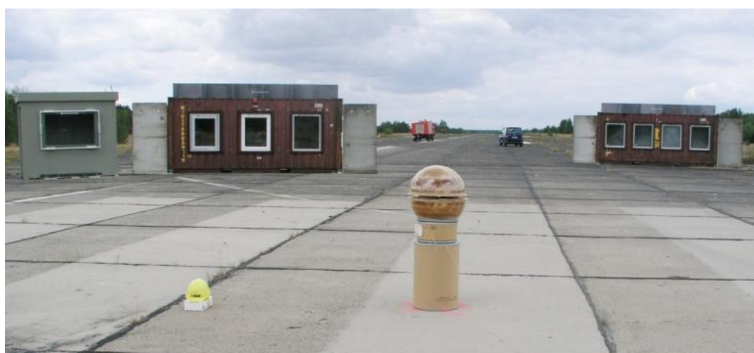
Figure 8: Typical arena test set-up for rating window systems.
